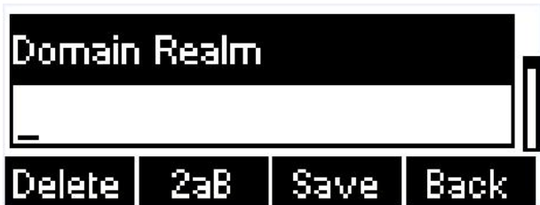
Figure 17 - Configure SIP Realm/Domain
