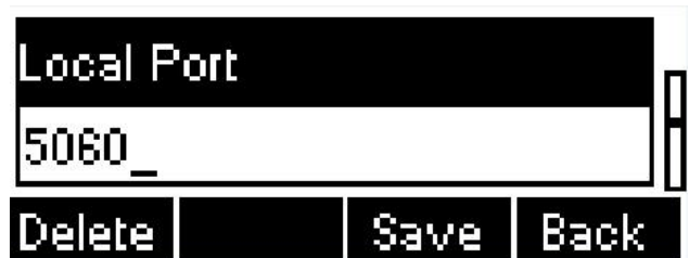
Figure 22 - Configure Local Port
