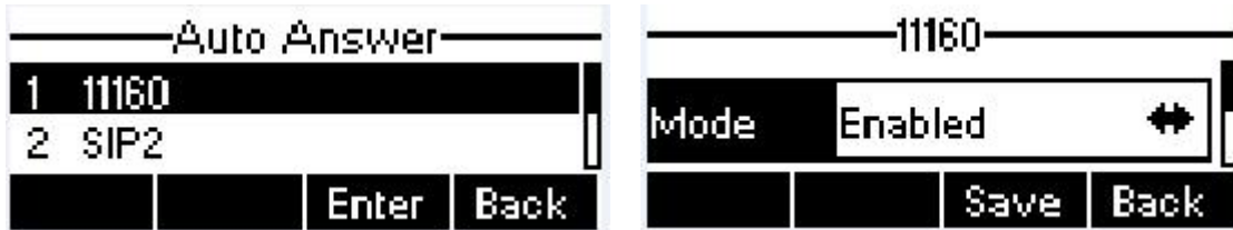
Figure 58 - Configure Auto-answering on Line1
