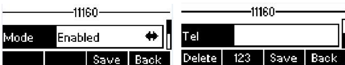
Figure 55 - Configure the Voice Message Number
