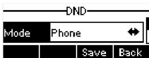
Figure 57 - Configure DND on Line
