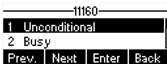
Figure 61 - Select Call Forward Type
